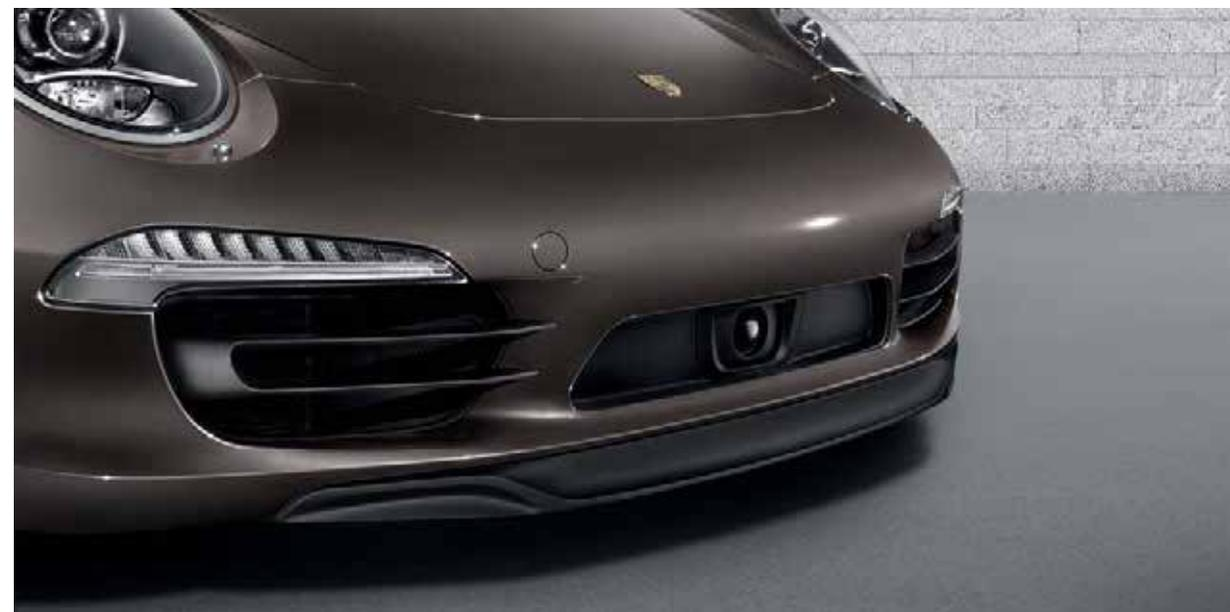
Radar sensor of Adaptive Cruise Control
