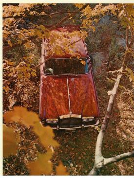
1. The Silver Shadow is the first Rolls-Royce to have monocoque construction. Its body and chassis are all in one piece. This has four important advantages.
