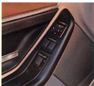
**C**onvenient power windows are standard on all Thunderbirds. Controls are located in the door panel armrests for easy identification and comfortable operation. See page 27 for availability of dual electric remote mirrors and power door locks shown also.
