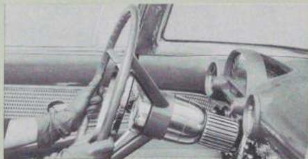
New deep-center Lifeguard steering wheel acts as a cushion to protect the driver's chest from the unyielding steering column, should he be thrown forward in an accident. Wheel position is telescopically adjustable.
