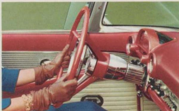
New deep-center Lifeguard steering wheel acts as a cushion to help protect driver from the unyielding steering post, should he be thrown forward in an accident. Wheel position is telescopically adjustable.
