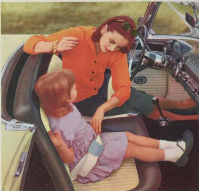
New optional Ford seat belts help hold you and your passenger firmly in the seat in the event of an accident. Belts are securely anchored to reinforced, all-steel floor structure. They're easily adjusted or released with one hand. Lifeguard rear-view mirror and new optional Lifeguard sun visors give you extra protection against injury should an accident occur.
