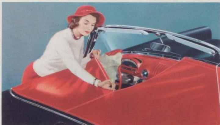
New optional color-keyed tonneau cover snaps on neatly and quickly. Protects driver and passenger compartment from dust, dirt and rain. Converts from one piece to two pieces in seconds. Simply unzip it and you can remove cover from driver's side.
