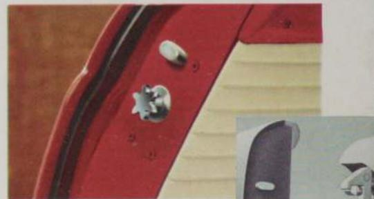
New Lifeguard double-grip door latches reduce possibility of doors springing open . . . give added protection against being thrown from the car in accidents.
