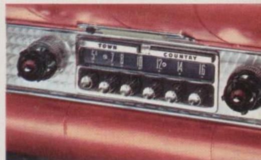
New Transistor-Powered Volumatic radio automatically tunes in stations in either direction on the dial. Also, it automatically "raises and lowers its voice" as car speed increases and decreases.
