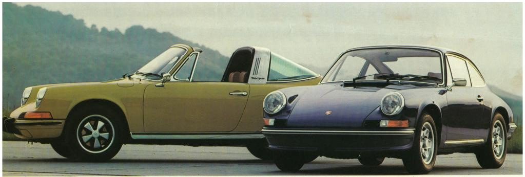
The Porsche 911 is obtainable either as a coupe or Targa model with three different engine specification versions available. Firstly, there is the 911 T with its two triple choke carburettors (virtually one carburettor per cylinder) producing 130 b. h. p. DIN or 147 b. h. p. SAE. Secondly, there is the 911 E, fuel injected producing 165 b. h. p. DIN or 185 b. h. p. SAE. Thirdly, there is the 911 S, also fuel injected, producing 190 b. h. p. DIN or 210 b. h. p. SAE.
