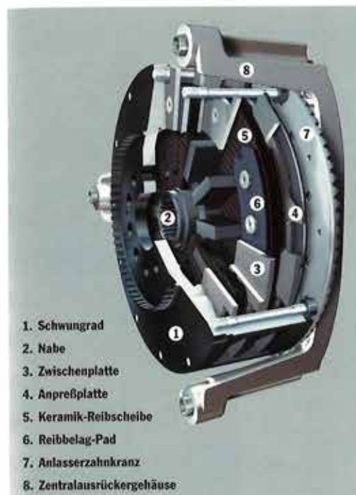
Porsche Ceramic Composite Clutch (PCCC)
